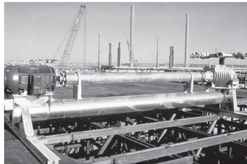
The heavy nature of the castings from which the couplings are machined usually makes the hot dip galvanized couplings acceptable in all but the more corrosive atmospheres. See page 19 for optional "all stainless" and carbon fiber drive shafts.
